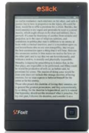
A FOUR-WAY controller (at lower right) on the eSlick turns pages.
